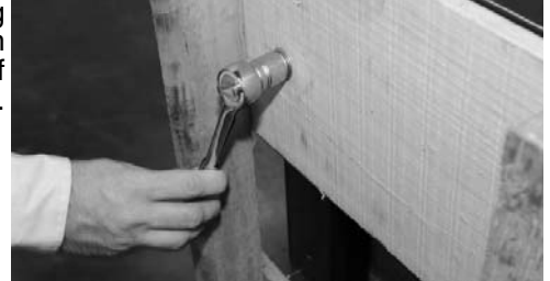
Removing skid from bottom of cabinet.
